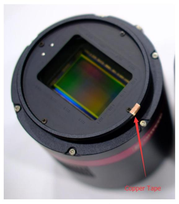
Typically the Copper tape is 65um an 100um. One piece of the copper type can generate about 20-30um adjust results.
