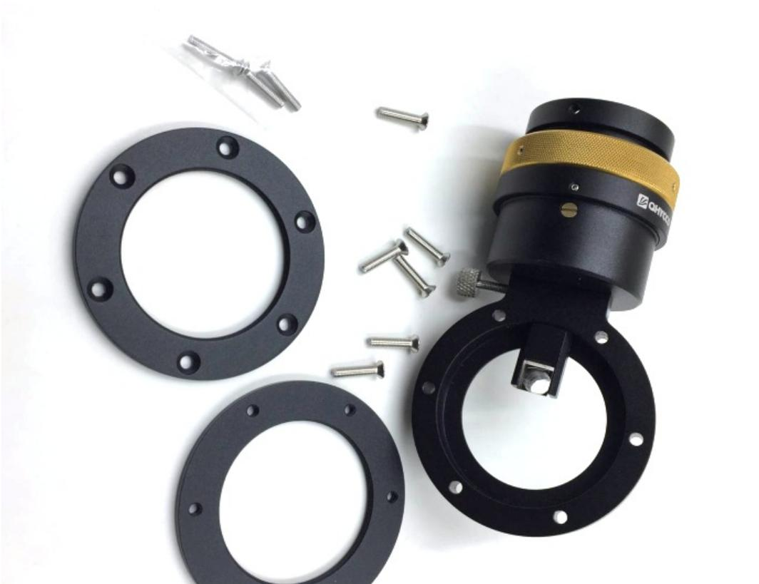
Put one piece on front of the OAG, one on back side of the OAG. Use six M3 screw to connect them. Normally speaking the one with M3 thread should be put in back side of the OAG. Now with the two piece thread adapter the total length is 16mm.
