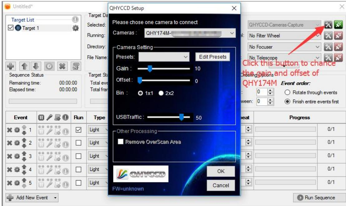
The next step is going to connect your filter wheel (QHYCFW2-M). Before you select QHYCCD Filter wheel as the filter and click the red connect button, you should also make sure you've connected QHY174M to filter wheel (QHYCFW2-M) with DIN4/RJ11 cable, you've plugged in the 12V power supply cable, you've installed the Filter wheel drivers, and the initialization of filter wheel has been finished.
