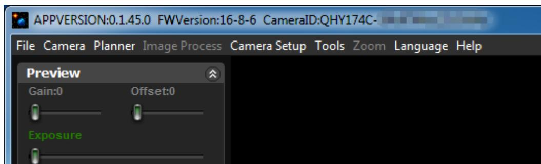
4. In Menu->Camera Setup, Click "Temp Control" and set the CMOS sensor temperature. You can enable the "Auto Control" and set the target temperature. For example here we set the temperature to -10C. The CMOS temperature will come to -10C very fast (in about 2-3minute). If you want to close the TEC, you can select "TEC OFF". If you just want to set the TEC power but not the temperature. You can select "Manual" and then set the percent of the TEC power.
