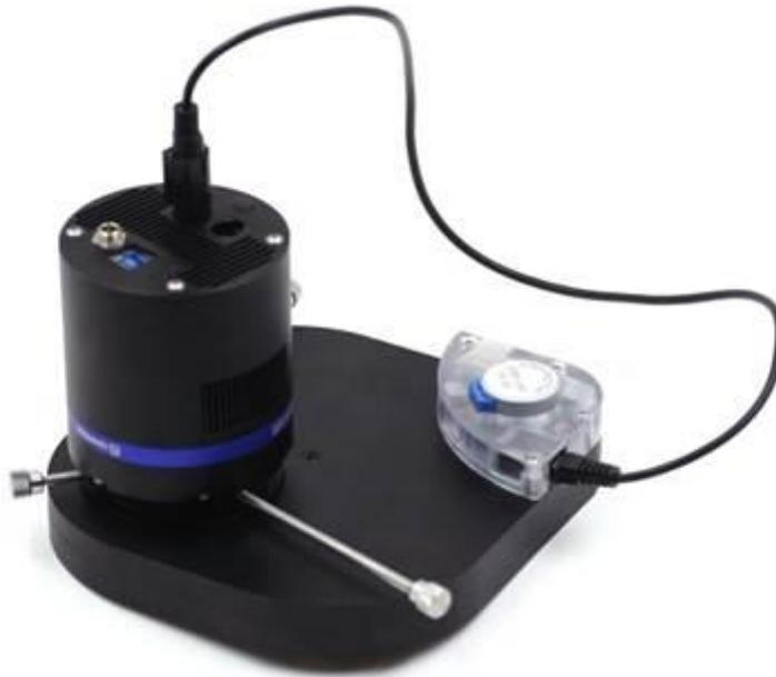
First, you need to stick QHY174M into QHYCFW2-M as shown in the picture above. Then you should screw those three bolts in. At the first time you screw bolts, you may find it a little bit difficult to screw in, in this case, please make sure that the bolts are pointing towards the center and apply a little bit more of force. Finally, you should connect your QHY174M with QHYCFW2-M by using DIN4/RJ11 cable, which is included in the box.
