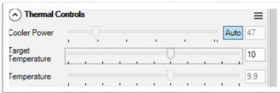
Basically, you can control the temperature of CMOS by either adjusting "Cooler Power" or clicking "Auto" and adjusting "Target Temperature". You can also see the CMOS temperature at lower-left corner of the software.
