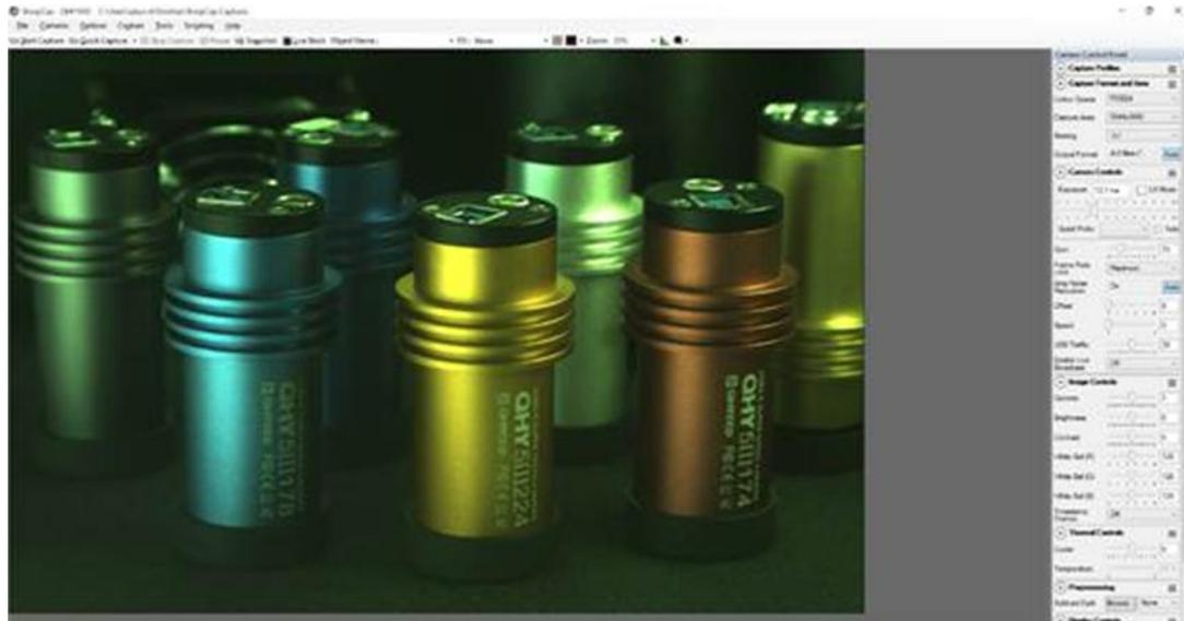
For color camera, SharpCap will show the WB Red/Green/Blue progress bar. Since the color balance is the ratio between Red to Green and Blue to Green. You can fix the Green color to 128 and adjust the Red and Blue.
