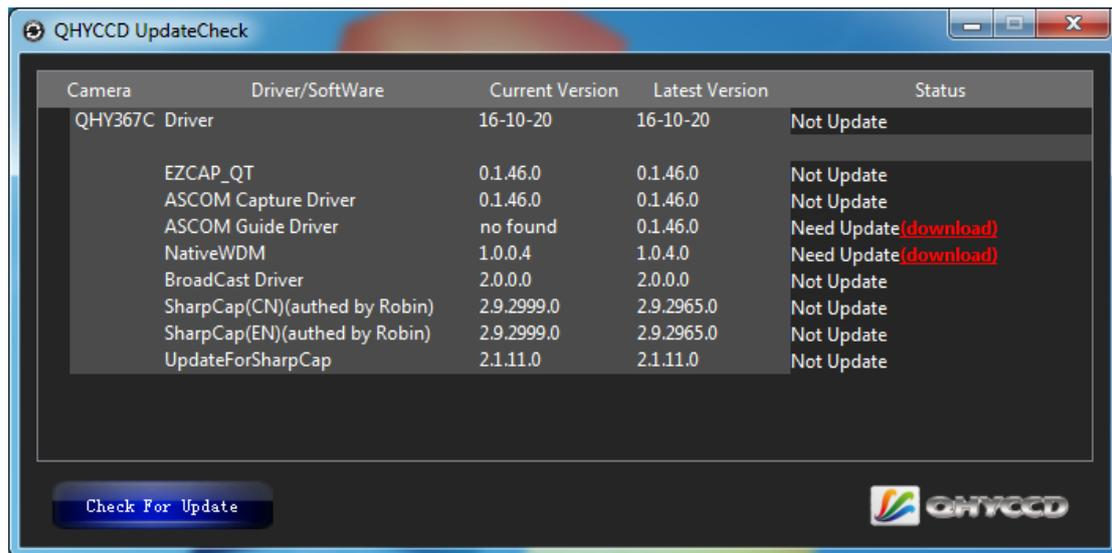
Note that after you downloading and installing the new drivers by using this software, be sure to pull the USB cable out and then plug it in to enable the new drivers.
