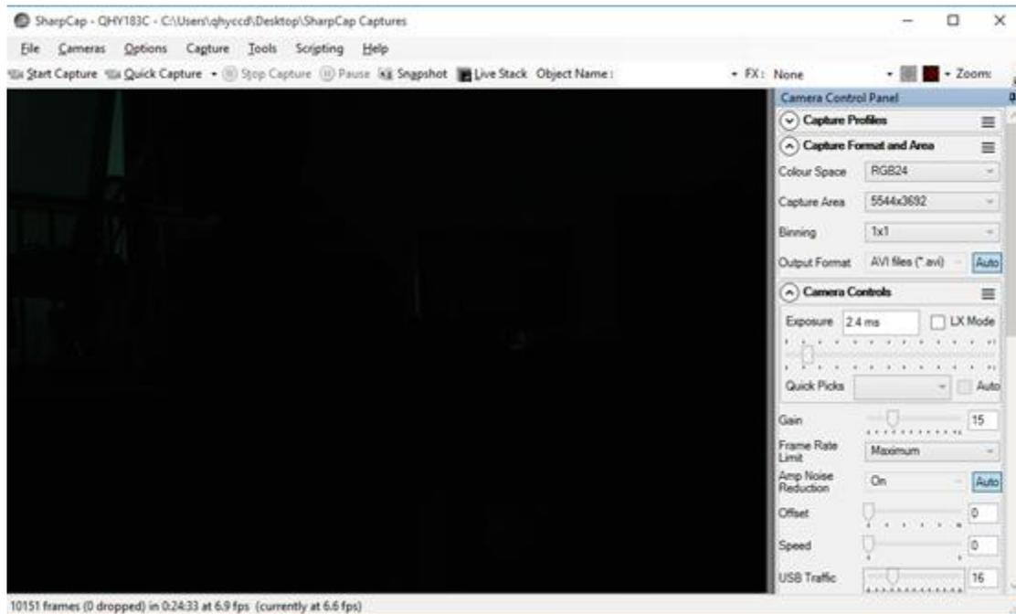
3. If you have started the SharpCap before connecting camera to your PC. You can click menu->cameras->rescan for cameras to search the camera and check on the camera name (QHY183C in this case).
