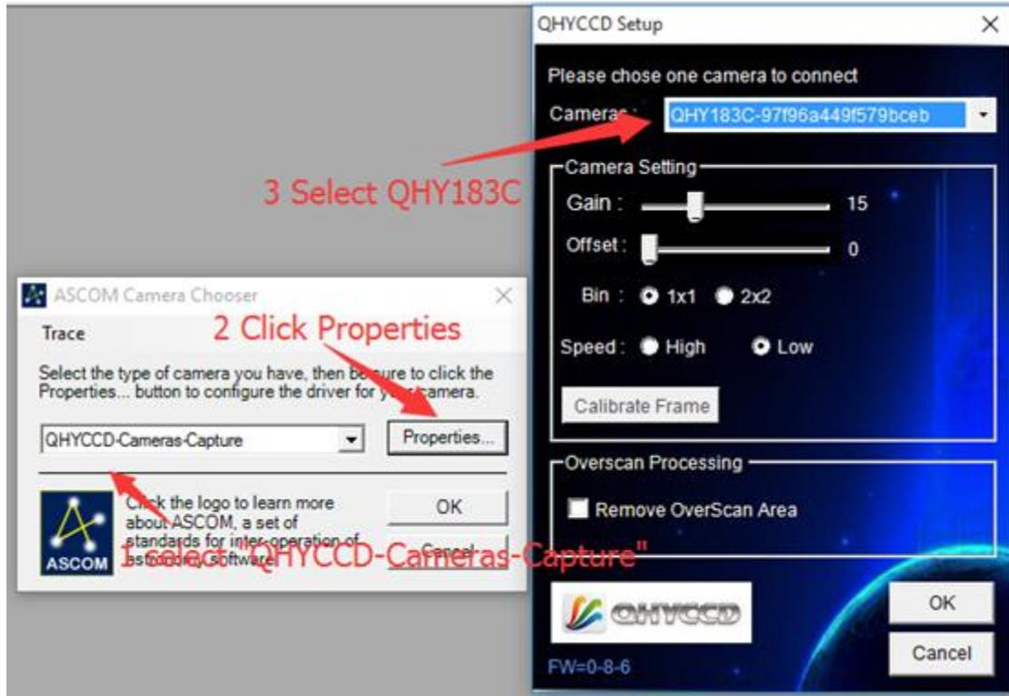
Normally, you can set the gain=1 and offset=10 to start. The speed and overscan calibration options are no use to QHY183C.
