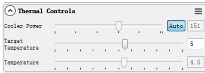
Basically, you can control the temperature of CMOS by either adjusting "Cooler Power" or clicking "Auto" and adjusting "Target Temperature". You can also see the CMOS temperature at lower-left corner of the software.
