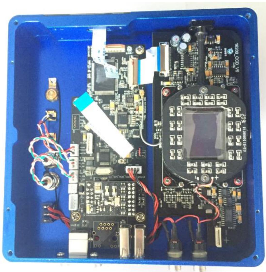
The CCD chamber is connecting with the silicone gel tube socket by a rubber pipe. Remove the two screw for the silicone gel socket.
