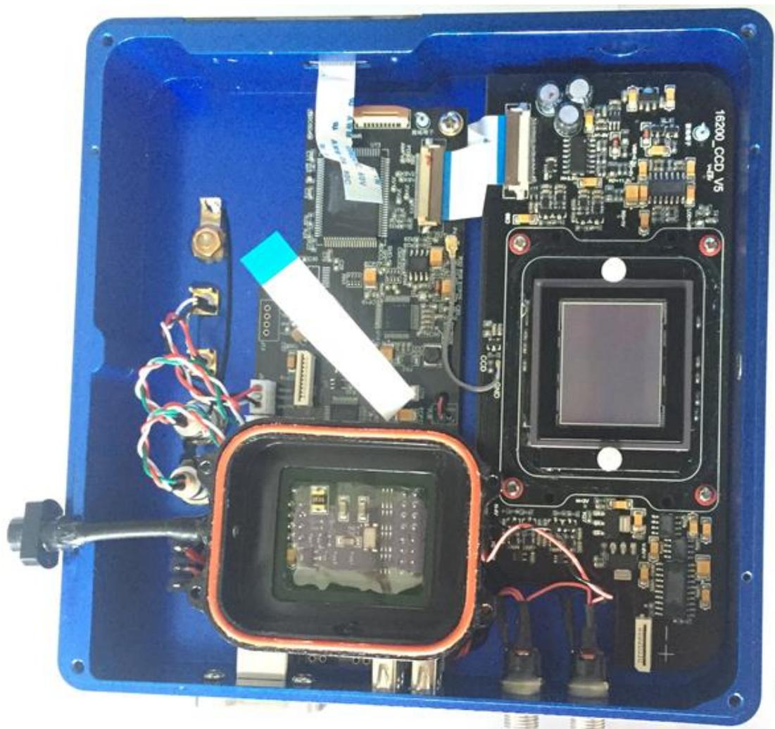
The CCD sensor has the AR coating. Please clean it carefully by using the lens paper or another professional tools (like the DSLR sensor clean tools)
