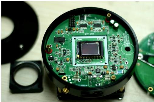
Clean the CCD surface carefully. The CCD surface has an AR (Anti Reflection) coating, so care must be used when cleaning. For dust or fibers, a blower bulb should be used, and alcohol or similar cleaning agent with a very soft lint free cloth (Micro Fiber cloth) for hard to remove spots. Use single sweeps while cleaning, turning over and using a clean side on every sweep of the glass.
