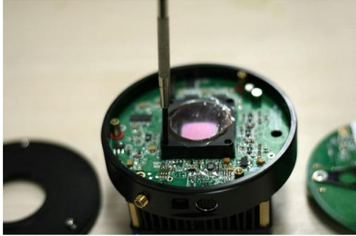
4. Lift the CCD chamber case of the main board
