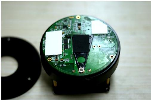
3. Remove the upper PCB board by gently lifting a little bit at a time around board.
