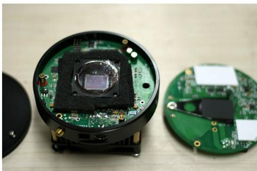
3. Remove the four screws of the CCD chamber (Chamber will need to be re gassed if you proceed)
