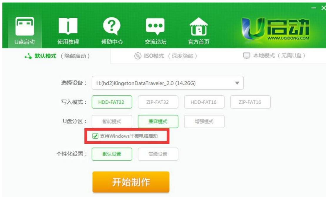
Use the default setting but make sure that the "支持 Windows 平板电脑启动" checkbox is checked as shown in the picture above.
