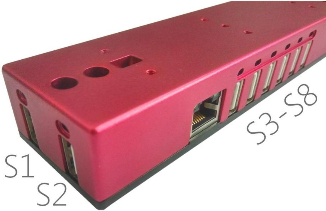
S1-S6 are controllable, which means you can turn them on or off separately by using the built-in software, AstroComputerCtrl.
