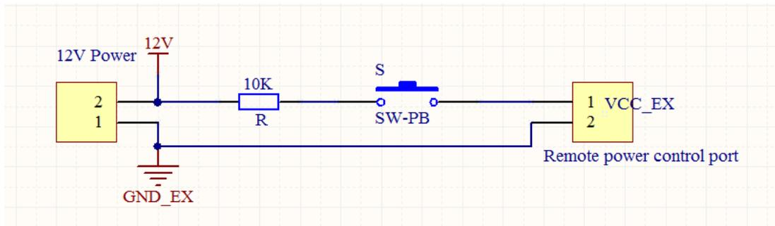
**Drawing of remote power control port application circuit**
