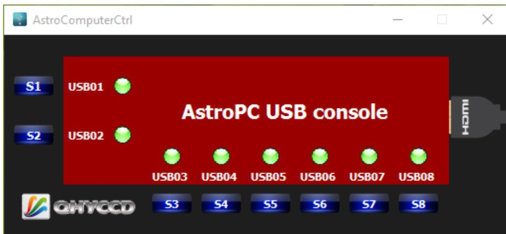
You can turn some USB port off by clicking its respective button, and the green indicator will turn to white. For example, we can turn USB06 off by clicking "S6" button.
